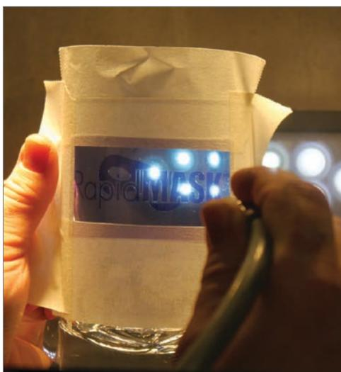
Photoresist protects surfaces that shouldn't be sandblasted while exposing surfaces that should be.
