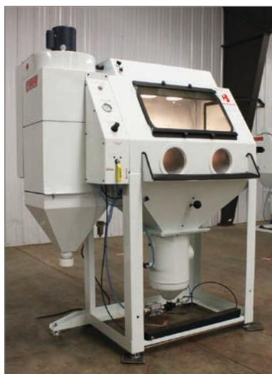
This is an example of a direct-pressure system for sandblasting.
