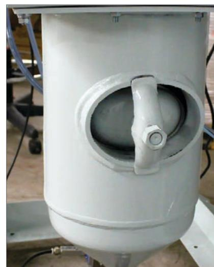
This is an example of a pressure-pot sandblasting system.
