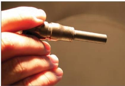
Direct-pressure sandcarving machines typically use the standard  $\frac{3}{32}$ -in. nozzle, using 5–6 cubic feet of compressed air per minute during the sandcarving process.
